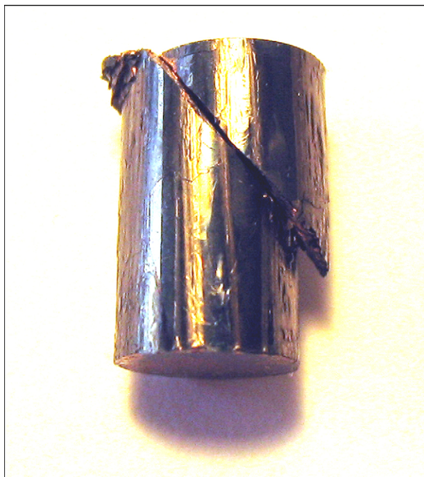
Fig. 7. Compression specimen fractured at a shear band at 45°.
